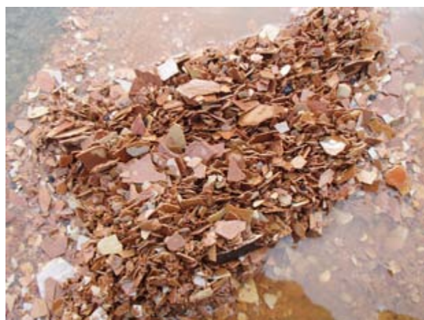
Picture showing scale chips from a 14" Brine Water Pipeline
