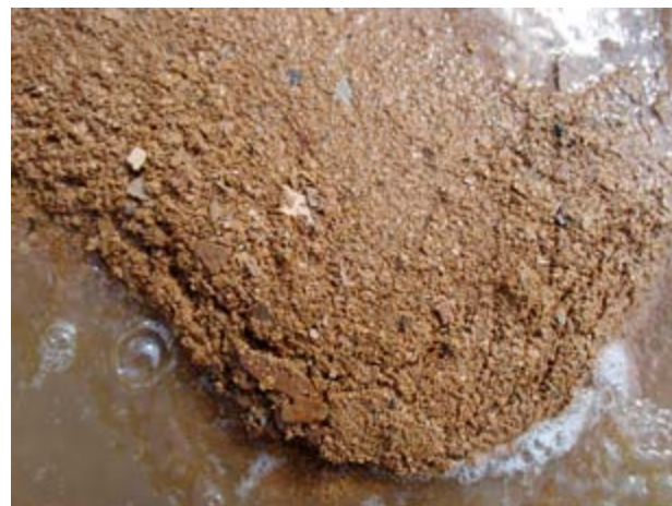
Picture showing crushed scale chips after the third MCT cleaning run in a 14" Brine Water Pipeline
