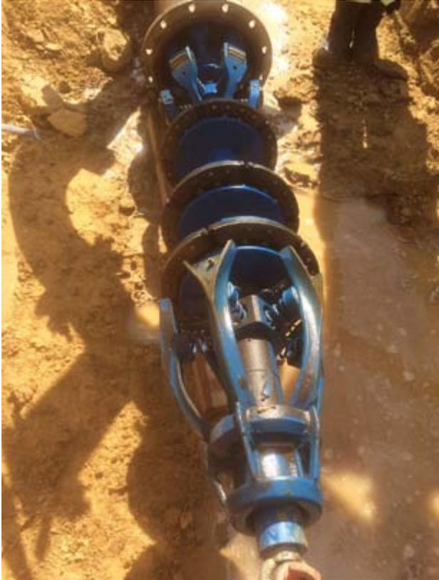
*Pulling out a 12" mechanical cleaning tool*
