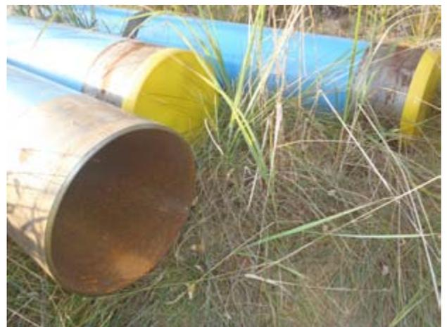
*Bad storage of pipelines leading to corrosion and rust*
